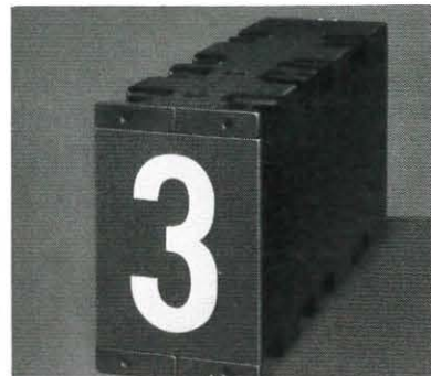
80 —Large screen unit suited for annunciator applications such as factory call systems and production control. 3 3/8" character height can easily be read at 100'. 160° viewing angle.
